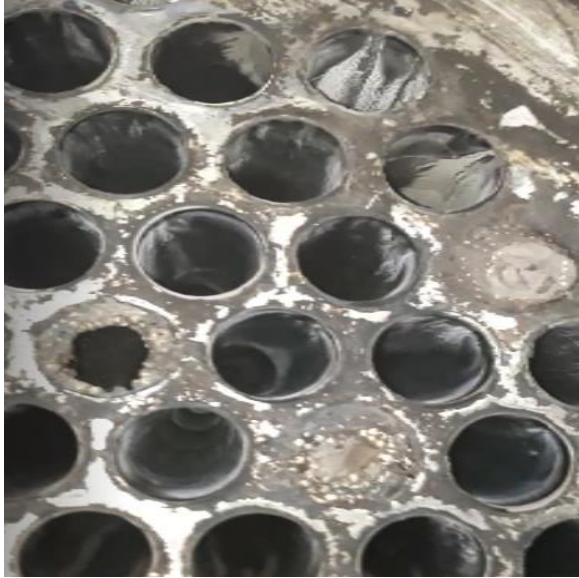
Figure 5: Inspection of the heat exchanger tubes of the first effect after 400 hours of operation
