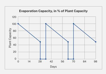
Evaporation processes are crucial across industries, from chemical processing to food and beverage production. However, scaling, fouling, and other contaminants can hinder your evaporator's performance, leading to increased energy consumption and decreased production capacity. As a result, regular cleaning and maintenance are necessary to prevent fouling and ensure the efficient and desired operation of evaporators.
