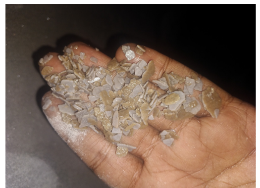
Picture 2 : A visual representation of the fouling layer found in the first two effects
