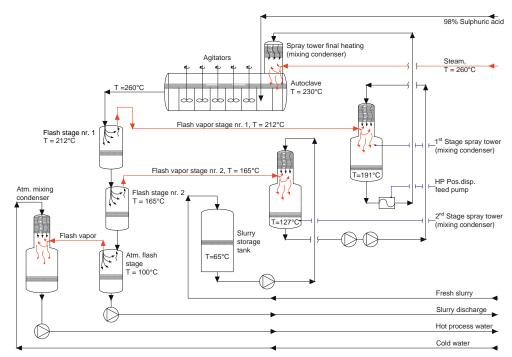
▲ Figure 1. HPAL for laterite nickel employing direct heat transfer.
