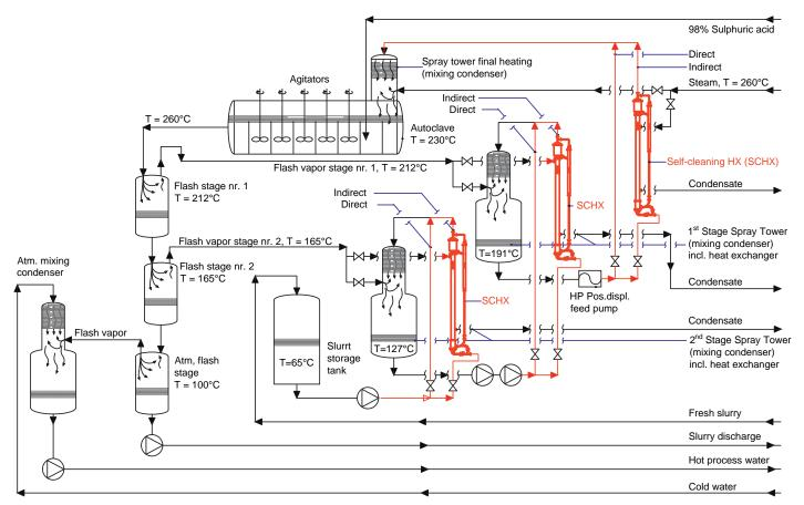
≈ Figure 3. HPAL for laterite nickel employing direct heat transfer revamped into indirect heated configuration.
