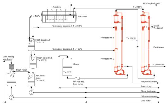
≈ Figure 2. HPAL for laterite nickel with indirect heat transfer (self-cleaning heat exchangers).
